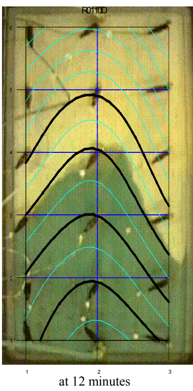
Figure 5: Comparison of actual and reconstructed flow front progression.
